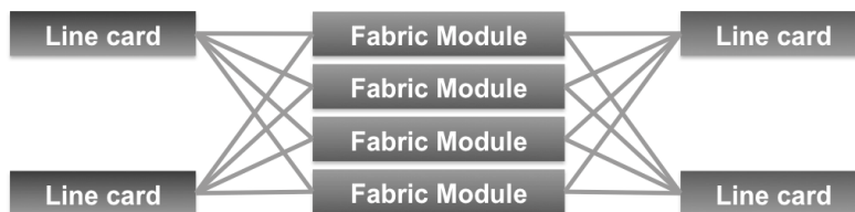
Figure 4: Advanced CLOS Architecture
